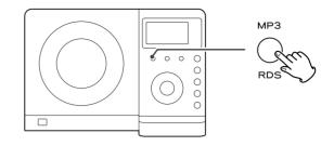
During playback of an MP3 disc, press the MP3 button for more than 1 second. The information about the current track is displayed as follows:
